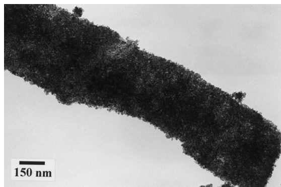
Fig. 4. Transmission electron micrograph of CZ68 treated at 923 K showing a complete morphological homogeneity.
